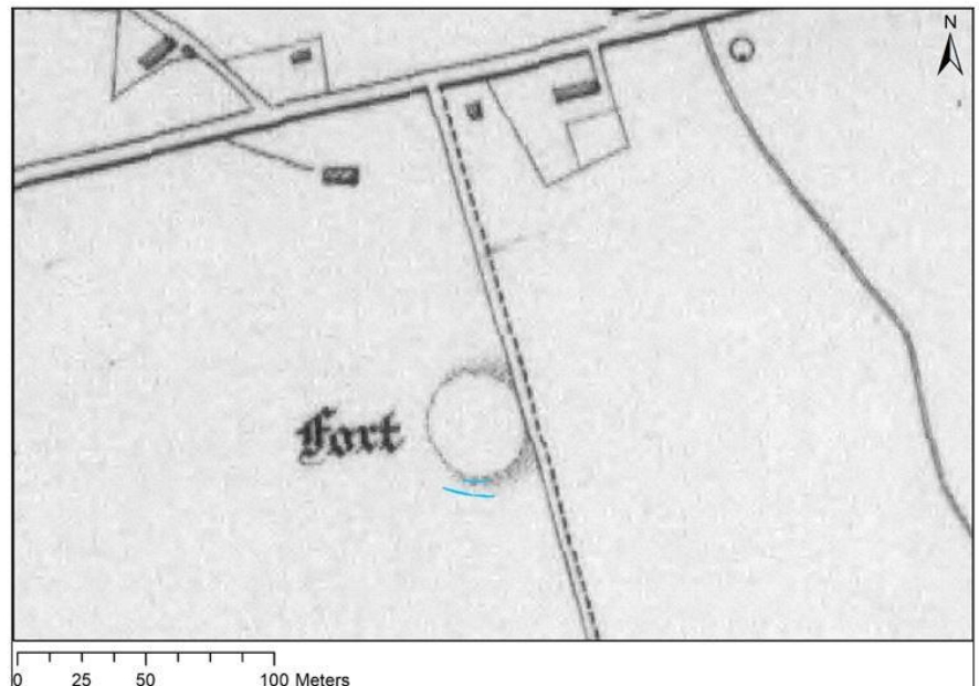
Resistivity anomaly overlaid on 1 st Edition Ordnance Survey six-map sheet (c.1830). Note that an outer enclosing feature was detected in the survey. This element is not recorded in the mid-19 th century map, and it suggests this was once a more complex monument.
