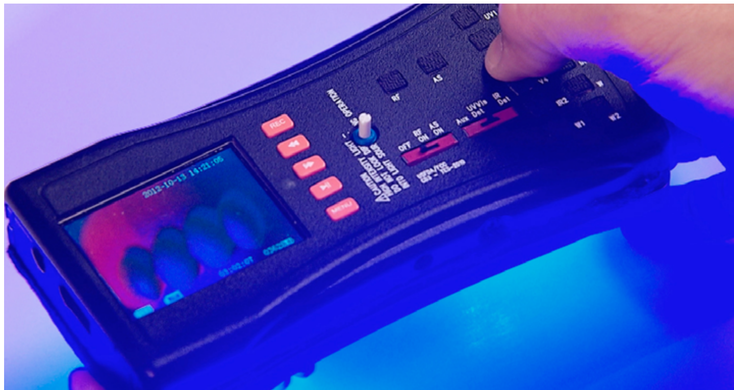
Authentic and counterfeit drugs being screened by CD-3, a small portable device invented by FDA scientists © U.S. Food and Drug Administration.
